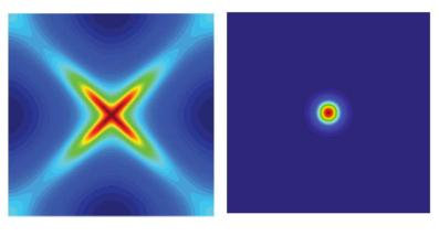
Figure: Fracture simulation in thick plate using Phase field damage model under transverse (a) static load (b) dynamic load
